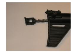
Remove the buffer from the recoil spring and install the buffer cylinder with the stainless steel disk facing the rear, toward the buffer.
